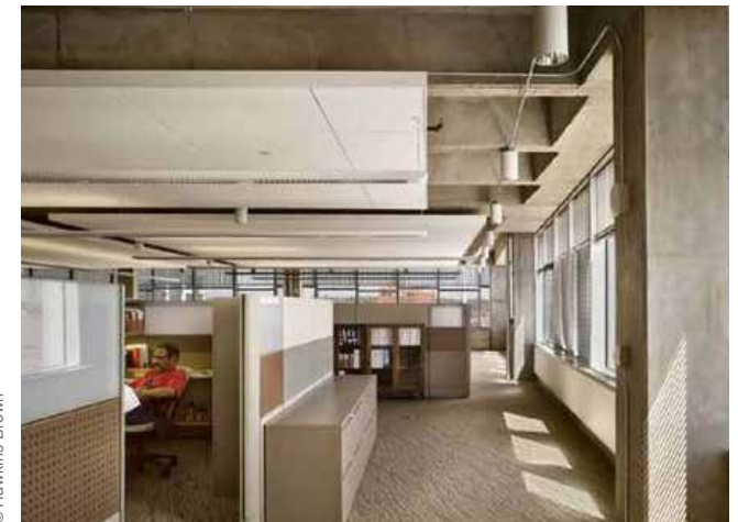
High thermal mass, exposed concrete finishes at EPA headquarters, ZGF Architects, Denver
