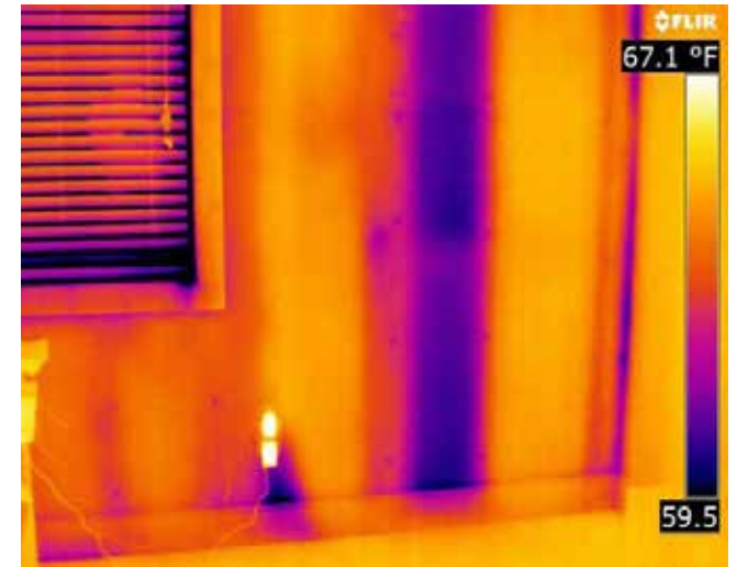
Thermographic surveys can be used to check quality of construction and identify defects such as areas of missing insulation
